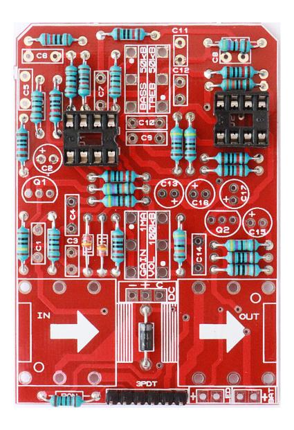
First of all place the pin header and then the IC sockets (without the ICs).
